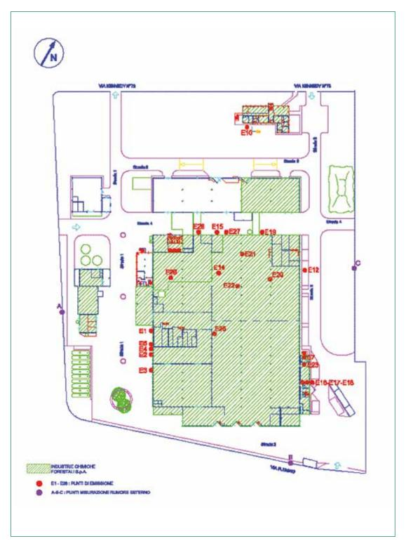
Fig. 05 – Plant layout showing emission points (Scale 1:1600)
