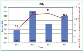
Emission reduction of VOS and CO<sub>2</sub> are attributable respectively: -to a lower VOS output because the post combustor provides the total combustion, while the active carbon filters restraines only a part of VOS emitted and -to a decrease in gas consumption in the using of impregnator caused by a little decrease in the production of the impregnated fabric.
