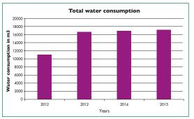
The increase of water in the plant, in the last three years, is imputable to an increase of water-based adhesives production and to an increase of water used by the post combustor. Even if a part of the water used in the production is also used to wash the machine, it is observable è little increase in the consumption of water in the 2015. This increment is caused by an increment of water-based adhesives production.
