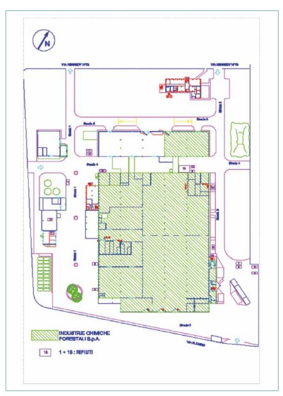
Fig 06 – Plant layout showing collection points for separate waste collection (Scale 1:1600)
